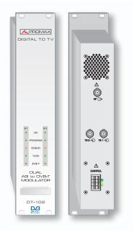
The **DT-102** (dual) modules are COFDM modulators compatible with DVB-T standard. They have TS-ASI input and RF output in the UHF band and are agile in frequency and output level. Inputs can contain services in all sorts of formats: SD, HD, MPEG-2, MPEG-4, etc.
